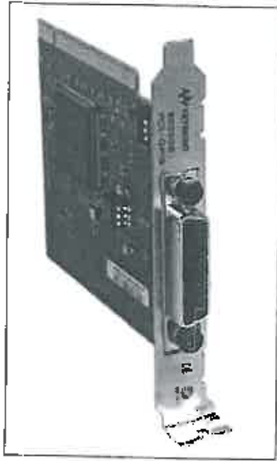
82350B PCI high-performance GPIB interface card
